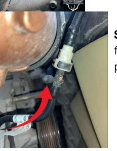
**Step 14:** Disconnect vacuum line from T fitting, this can be found below the intake plenum on the front side of the engine.
