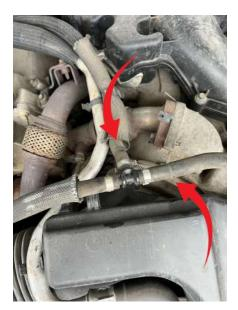
**Step 17**: Join the two hoses that are shown with the supplied barb fitting
