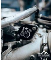
**Step 13**: Install provided EGR outlet block off plate, reusing factory hardware
