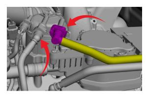
**Step 2**: Disconnect both fuel lines from fuel filter as shown
