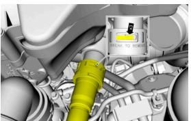
**Step 3**: Cut rubber sleeve off of crankcase vent oil separator outlet house & disconnect the hose.
