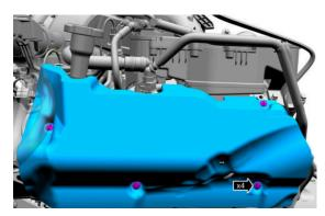
**Step 4:** Remove engine sound shield.
