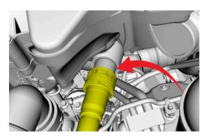
**Step 8**: Install the provided rubber cap in place of the hose that you removed earlier.
