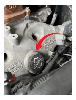
**Step 6**: Install supplied block off plate.
