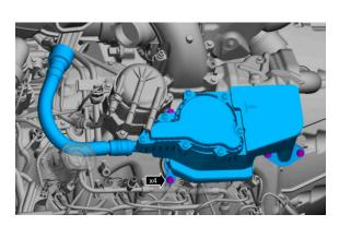
**Step 5**: Remove the crankcase vent oil separator bolts and then remove the whole assembly with the hose.
