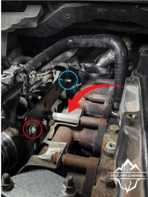
**Step 19:** Install provided mounting bracket with supplied standoff hardware (red arrow), attach coolant hose assembly (red circle) and back pressure sensor (blue circle).
