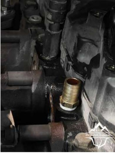
**Step 16:** Remove factory coolant fitting and replace with supplied barb fitting. Make sure to cover threads with teflon tape or thread sealer.
