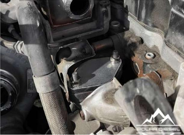
**Step 13:** Install front plate reusing factory hardware & gasket.
