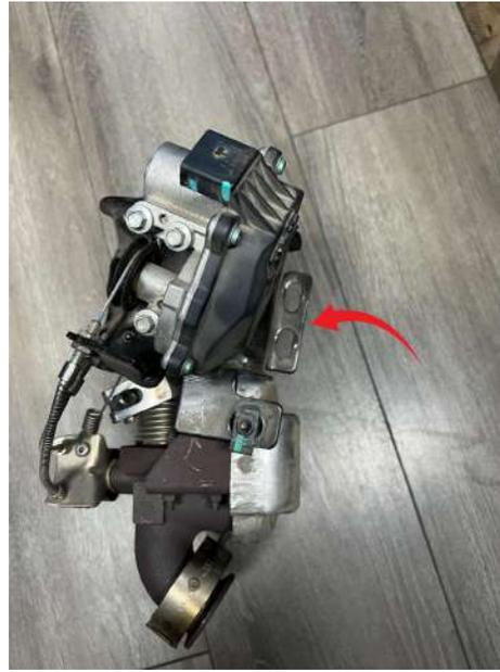
**Step 8:** Remove 4 bolts for the EGR bypass valve bracket and V-Band clamp that connects to the EGR cooler and move assembly off to the side.
