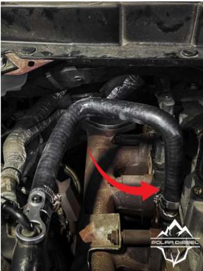
**Step 18:** Install provided coolant hose and trim to fit to provide clearance for CCV sensor.
