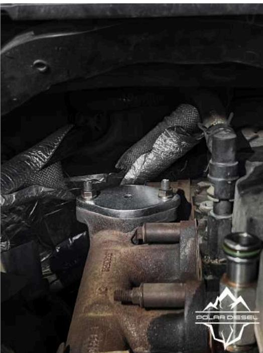
**Step 15:** Install rear plate reusing factory hardware and gasket.
