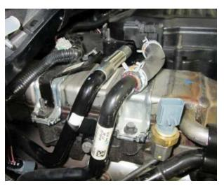
**Step 2**: Follow that same hose down and remove hose clamp(s) that are down towards the turbo. Pull the hose out.
