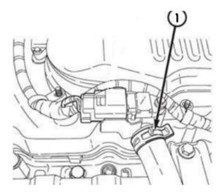
**Step 1**: Remove hose clamp off the vent hose that is attached to the valve cover.
