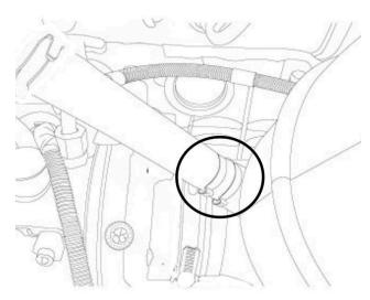
Step 3: Press in the provided plug to the lower hose that was connected to the turbo inlet and reinstall hose with the plug with provided hose clamps. If your truck is a 2019+, cut the factory hose near the compressor housing and install the provided plug.
