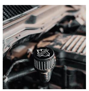
**Step 4**: Install the provided filter with 90 degree hose to the valve cover where you previously removed the vent tube using provided hose clamps.
