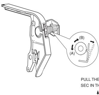
PULL THE THREAD AT THE SPEED OF 110 MM/ SEC IN THE DIRECTION OF ARROW
