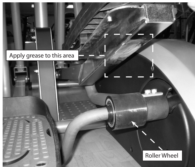
Correct Grease Application
