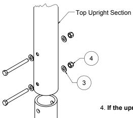
4. If the uprights are spliced, assemble the uprights with the splice tubes.
