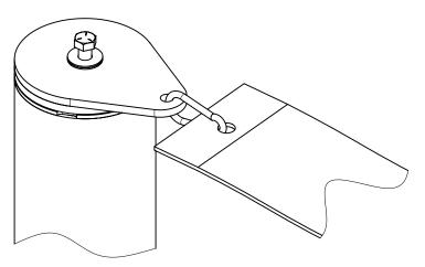
Install the flags onto the tops of the uprights BEFORE installing the uprights onto the crossbar.
