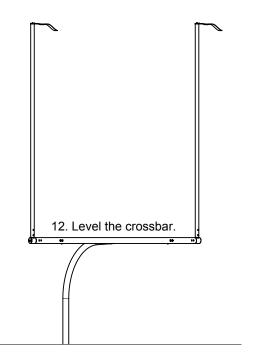
11. Install the second elbow joint and upright the same way as the first one.
