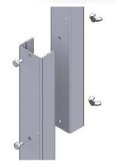
Align the holes in the middle upright with the holes in the bottom upright and secure with thumb screw and wing nut. Repeat for top upright.
