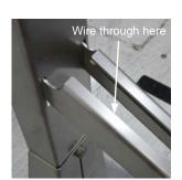
Secure unit to a sturdy surface with the c-clamp. Hang the hammer over the handle holder. Insert the wire stretcher over the hammer wire into the slots in the bottom upright. Push down to straighten the wire. If necessary, put the spacer between the ball and stretcher to straighten the wire.
