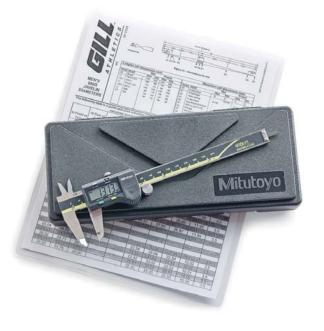
Use the digital caliper and included diameter chart to check the diameter of the javelin at each point defined by rule. Chart is laminated to allow common measurements to be filled in on the chart with a grease pen.
