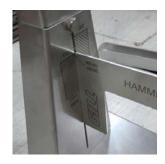
Slide the hammer square in the track up against the bottom of the ball. Read the scale on the base connector to see if the implement is within rule.
