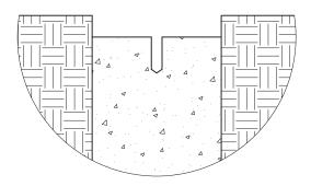
With the threaded opening pointing up, insert the anchor into the hole. Tap it down with a hammer.
