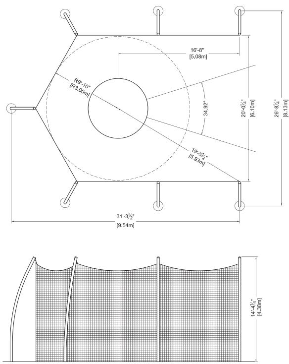
The 9020 Heavy Duty High School Discus Cage, consists of seven, 14' tall, rolled aluminum net poles with ground sleeves, a vinyl coated net support cable to reduce net sag, and a weather treated nylon net. Hinged net arms, at ground level, hold the net in place at the front of the cage. The poles are 4" OD, 0.218 wall, 6063-T6 aluminum tube. Each pole stands in a 36" deep ground sleeve. The net is 180 lb. test nylon which has been weather treated for extended service life.
