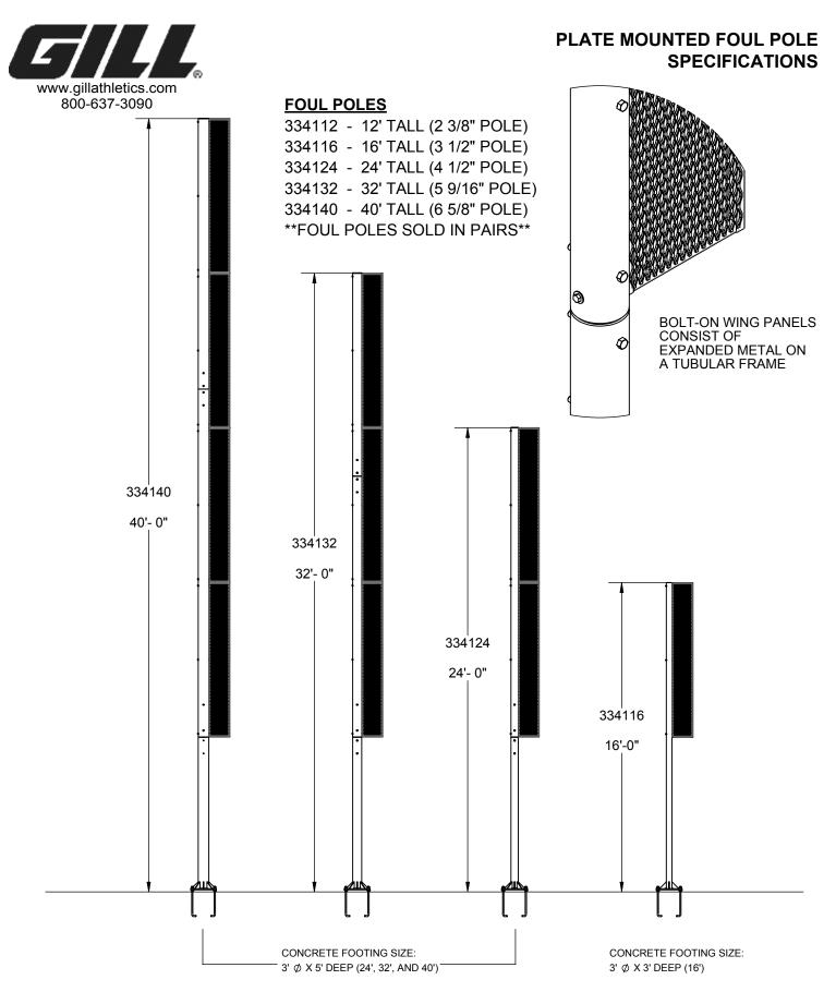
THIS IS THE MINIMUM RECOMMENDED FOOTING SIZE. INCREASE SIZE OF FOOTING AS REQUIRED ACCORDING TO LOCAL SOIL CONDITIONS, AND TO MEET LOCAL BUILDING CODES REGARDING MINIMUM WIND SPEEDS.
