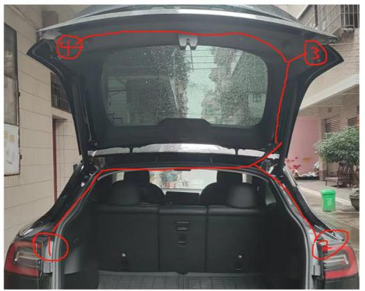
3.2 Connect the Full-Width Tail Light harness to run under the car leather strip
