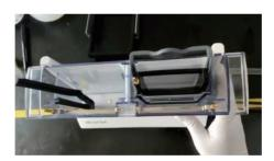
Take out the adaptor plate. User will find both sides of the adaptor plate have black color sealers. One side is longer and it is defined "the long side"; the other side is defined "the short side".
