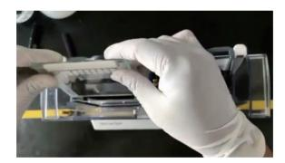
Install the cassette clamp, then the gel is successfully installed in the tank.
