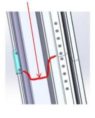
**2.**drill diameter 12mm holes on the wall tube, depth is 10mm stuff M12\*75 expansion plug into the holes and screw the wall tube on the wall by wood screw M8\*90.Don't forget do silicon sealant work at the gap
