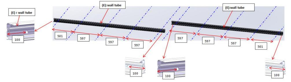
1.1 drill 5 pcs holes (diameter 12mm) on the wall tube .both end of wall tube has 100mm inward migration
