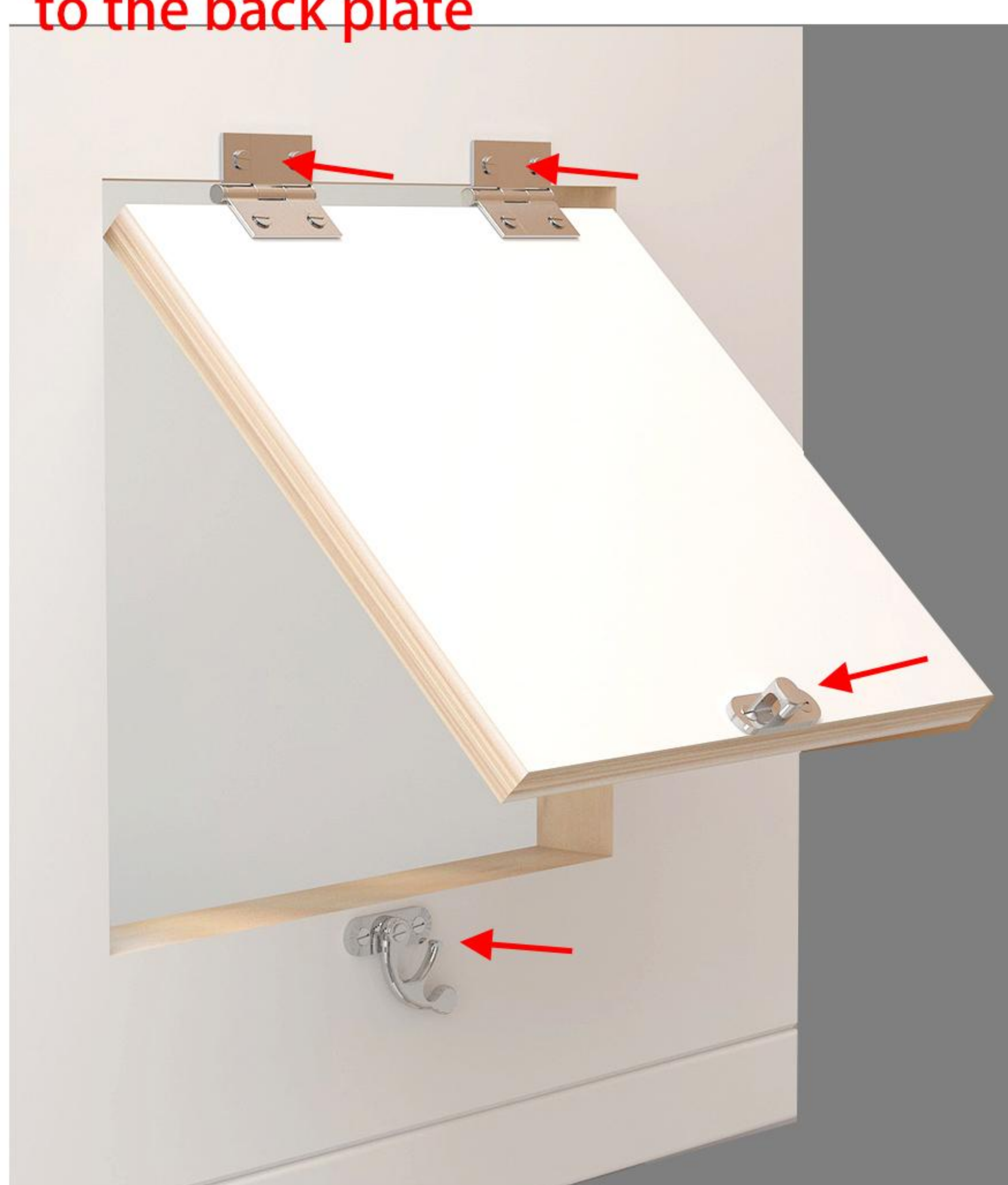
12: Install the access door and link it with a 1.5cm screw
