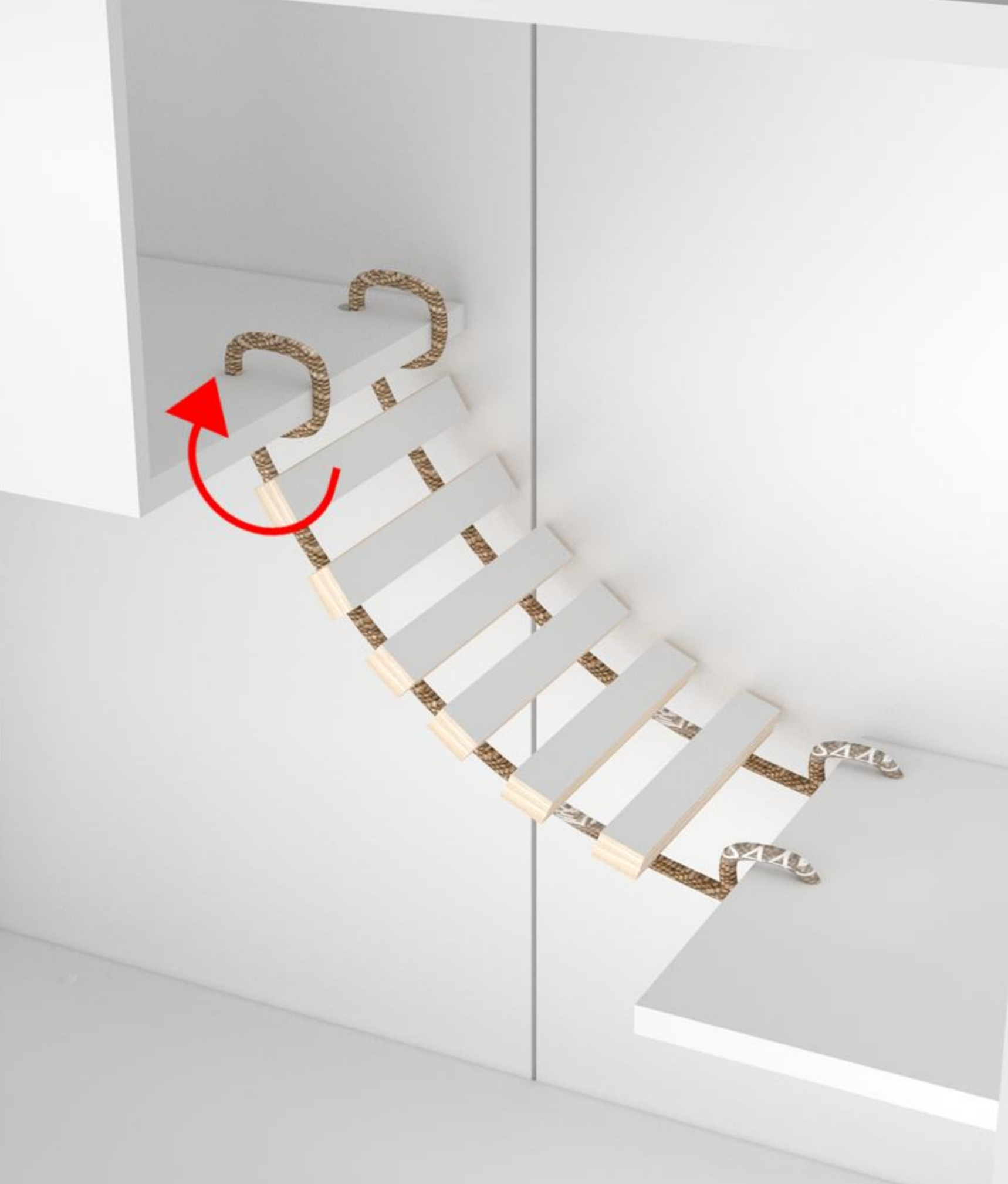
10. Install the suspension bridge, thread the suspension bridge rope from bottom to top through the corresponding hole position, and fasten it properly
