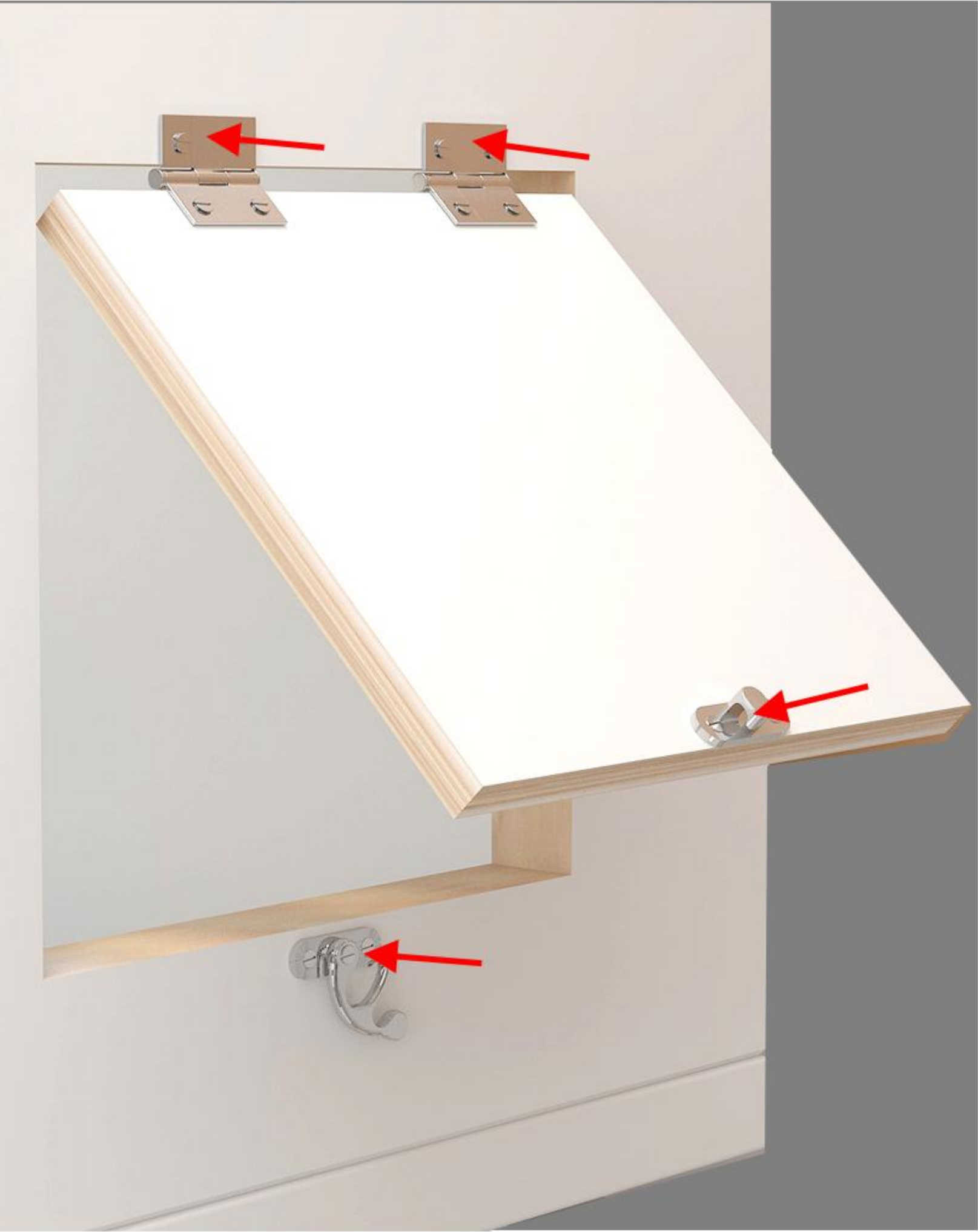
12: Install the access door and link it with a 1.5cm screw
