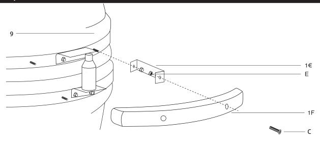
STEP 10 - To attach the handle (10) to the lid of the Kamado Grill (9) start by attaching 2x handle brackets (11) using the 2x pre-attached bolts and dome headed nuts. Attach the handle (11) to the brackets (10) using 2x bolts (C) and nuts (E).
