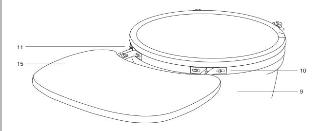
STEP 14 - Insert the 2x table hinge (15) into each of the table brackets (10 & 11).
