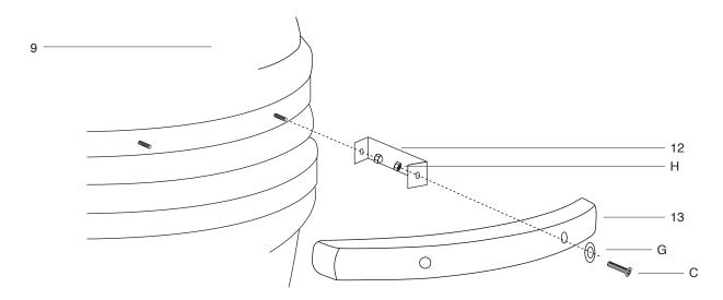
STEP 10 - To attach the handle (13) to the lid of the Kamado Grill (9) start by attaching 2x handle brackets (12) using the 2x pre-attached bolts and dome headed nuts. Attach the handle (13) to the brackets (12) using 2x bolts (C) and nuts (H).
