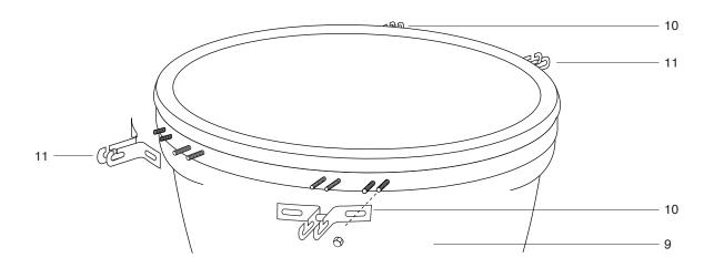
**STEP 12 -** Attach the 2x table brackets (10) to the Kamado Grill (9) using the 4x pre-attached bolts and dome headed nuts per bracket. Please note the position shown in the above diagram.
