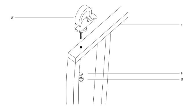
**STEP 1 -** Attach the four pre-threaded castor wheels (2 & 3) to each of the four brackets (1) by pushing them through the hole. Using an adjustable spanner secure each castor wheel with 1x nut (B) & 1x washer (F).
