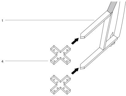
**STEP 2 -** To assemble the cart insert the two cross pieces (4) into one of the four brackets (1) from both the top and bottom.
