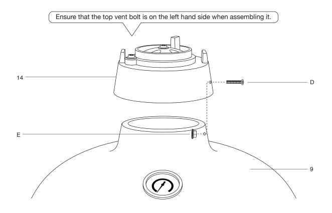
STEP 11 - To attach the top vent (14) to the Kamado Grill (9) place it on top and align both the bolt holes. Secure using 2x bolts (D) and nuts (E) Ensure that the top vent bolt is on the left hand side when assembling it.
