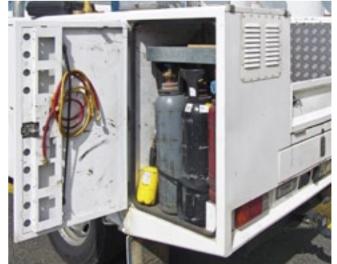
Purpose built sealed compartment
