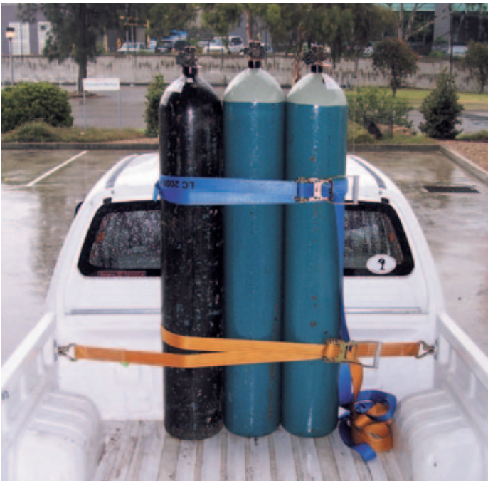
Example of correct positioning and restraining of gas cylinders
