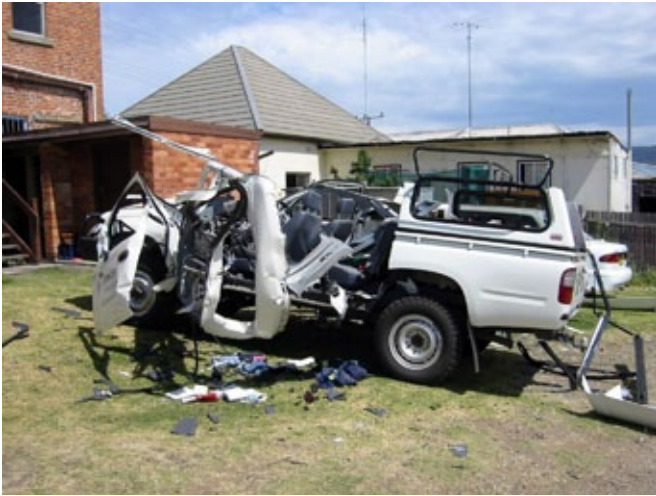
Vehicle explosion caused by a leaking flammable gas cylinder
