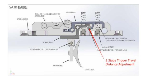
Clockwise tighten the screw to reduce the travel distance from the first stage to the second stage of the trigger.
