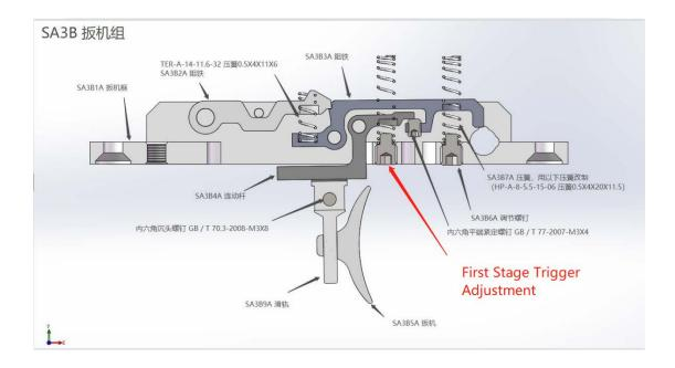
Clockwise tighten the screw to increase the trigger force of the first stage of the trigger.
