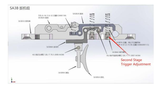
Clockwise tighten the screw to increase the trigger force of the second stage of the trigger.
