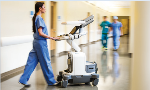
To reduce the time required for mobile scans, the system can be put to sleep in two seconds, and then moved to a new location, where it starts up in just seconds.
