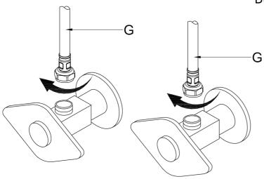
Thread the nut on the supply line onto the outlet of the water supply valve and tighten with a wrench. Do not overtighten.
