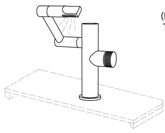
Turn on angle stops, turn the faucet on and check for leaks.
