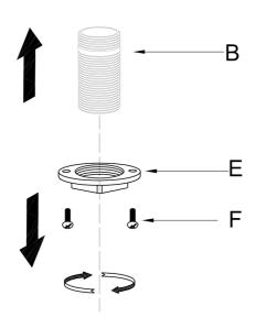
Shut off the water supply. Remove the old faucet. Clean the mounting surface. Remove mounting hardware (E & F) from threaded metal pipe(G).
