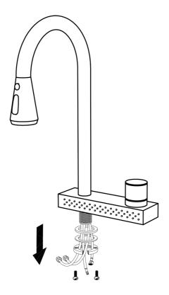
Shut off the water supply. Remove the old faucet. Clean the mounting surface. Remove mounting hardware (B~E) from the faucet.
