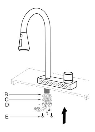
Pass the mounting hardwares (B~ E) through the water pipes in turn, install them on the faucet body and tighten.
