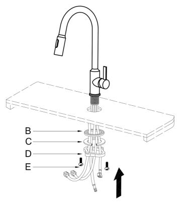
Pass the mounting hardwares (B~ E) through the water pipes in turn, install them on the faucet body and tighten.
