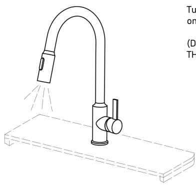
Turn on angle stops, turn the faucet on and check for leaks.
