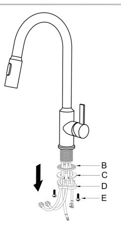
Shut off the water supply. Remove the old faucet. Clean the mounting surface. Remove mounting hardware (B~E) from the faucet.
