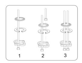
Step 4. Reattach the gravity hammer rope
