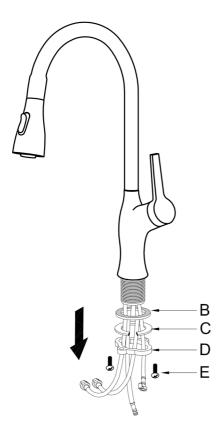
Shut off the water supply. Remove the old faucet. Clean the mounting surface. Remove mounting hardware (B~E) from the faucet.
