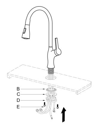
Pass the mounting hardwares (B~ E) through the water pipes in turn, install them on the faucet body and tighten.
