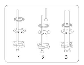
Step 4. Reattach the gravity hammer rope
