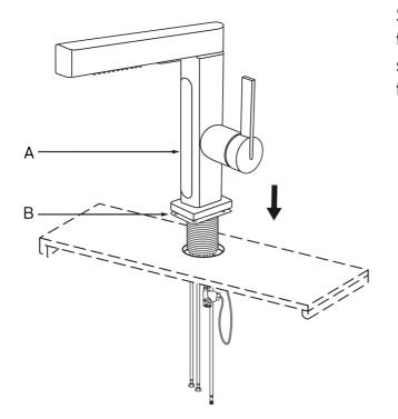
Shut off the water supply. Remove the old faucet. Clean the mounting surface. Thread the faucet through the hole and install it on the countertop.
