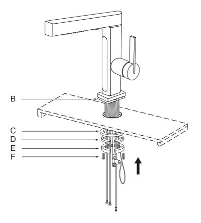
Install the mounting hardwares (B-F) in sequence according to the figure below, and fix the faucet on the countertop.
