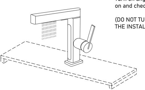
Turn on angle stops, turn the faucet on and check for leaks.
