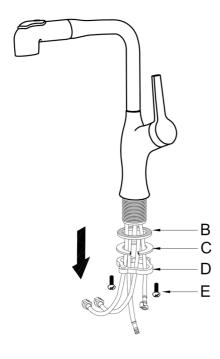
Shut off the water supply. Remove the old faucet. Clean the mounting surface. Remove mounting hardware (B~E) from the faucet.
