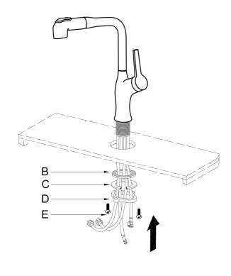
Pass the mounting hardwares (B~ E) through the water pipes in turn, install them on the faucet body and tighten.
