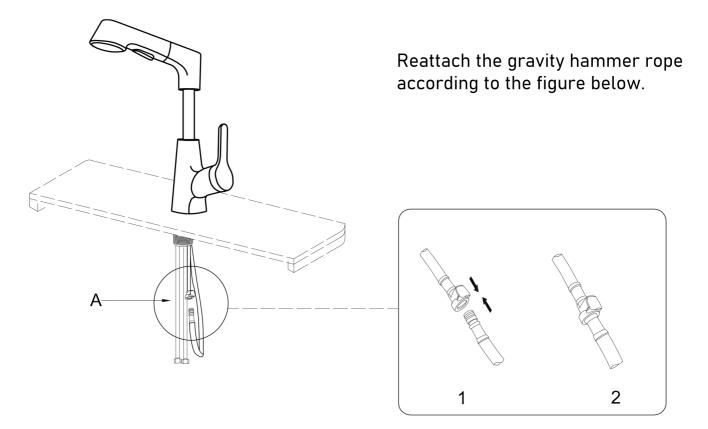
Step 6. Install gravity hammer
