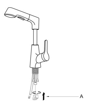
Connect the adapter of the gravity hammer rope to the faucet body.
