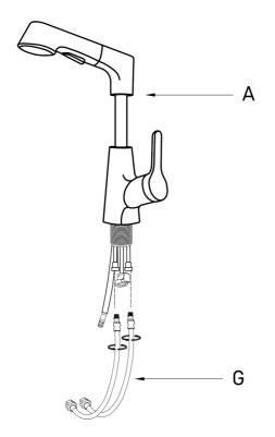
Swivel the hot and cold water pipes (G) into the faucet body (A).
