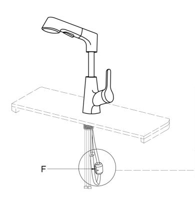
Operate the gravity hammer as shown in the picture below and attach it to the rope.
