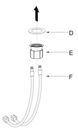
Install the hot and cold water pipes (F) through the mounting hardwares (E&D) and screw in tightly.
