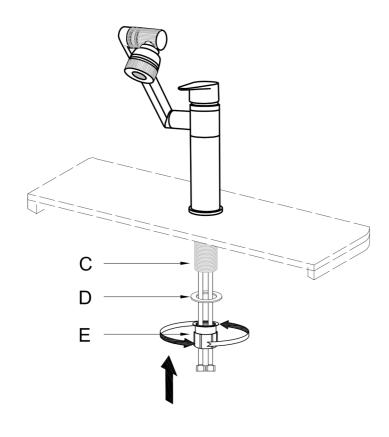
Install the mounting hardwares in sequence.
