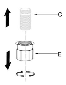
Shut off the water supply. Remove the old faucet. Clean the mounting surface. Remove mounting hardware (E) from threaded metal pipe(C).
