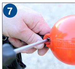
7 Using a Phillips head screwdriver unscrew float
