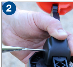
7 Remove pivot pin, dispose of spring cover
