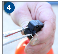
9 Remove spring retainer from float arm and remove damper spring
