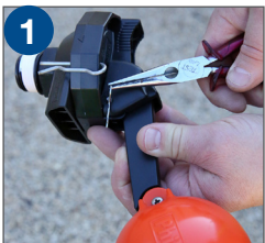
6 Remove small R-Pin that holds the pivot pin in place
