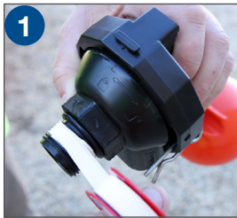
1 Apply PTFE tape in a clockwise direction
