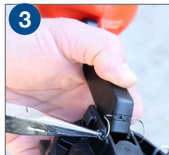
8 Unclip damper spring from cap
