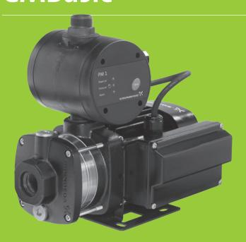
The BasicLine by Grundfos CMBasic is a compact booster pump designed for domestic and light industrial use. The booster unit consists of a Grundfos CM cast iron pump with stainless steel hydraulic components and PM1 Pressure Manager. The Pressure Manager allows the pump to start and stop automatically according to demand and protects the pump from dry running.
