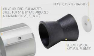
AS A HYDRAULICALLY OPERATED SLEEVE-TYPE VALVE, THE 800 SERIES CONTROL VALVE IS DESIGNED FOR VERSATILITY. THE BASIC BODY CAN BE EQUIPPED WITH SEVERAL DIFFERENT OPTIONS FOR CONTROLLING PRESSURE AND FLOW. IT'S ALSO ENGINEERED FOR EXTREMELY HIGH EFFICIENCY, RESULTING IN LOW PRESSURE LOSS AND HIGH FLOW CAPACITY.
