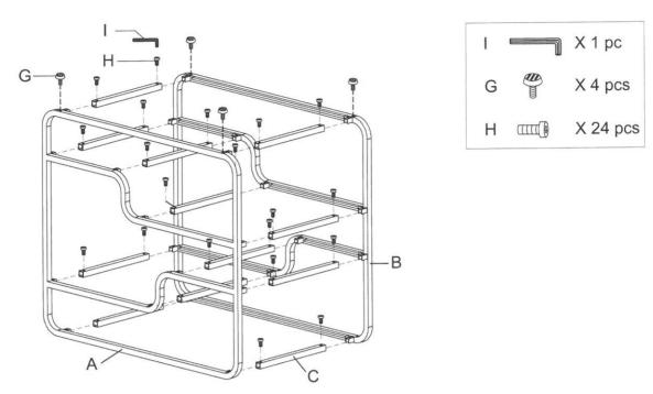
2 Upright the subassembly unit (A, B and C). Then place mirror shelf (D, E, F and D) onto each frame as shown in drawing.
