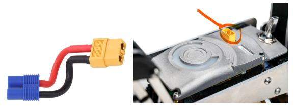
5. Plug the balancing cable into the power panel.
