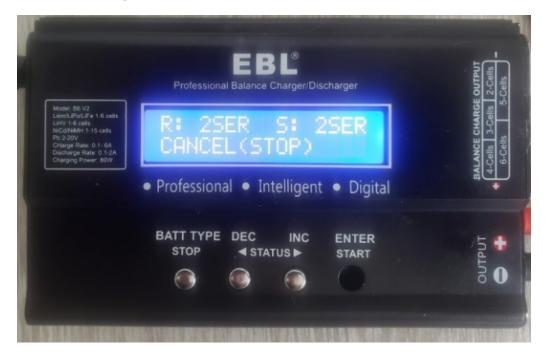
10. You may need to wait 30 minutes or more for the battery to fully charge. The battery charger will make a high-pitched sound to indicate a full charge. When the battery is fully charged, press the "Stop" button.
