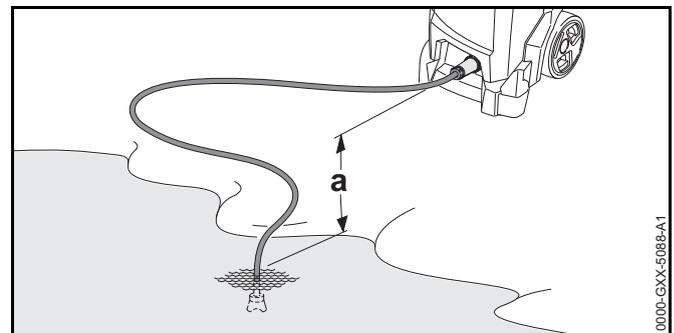
So that the water can be drawn in, the height difference between the pressure washer and the water source should not exceed the maximum suction lift (a),
