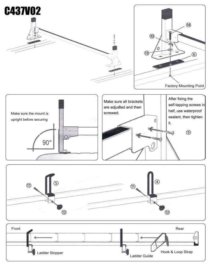
Please note: Each rack bracket already has a rubber seat on the bottom, and the bolt secures the bracket to the van using a sealing washer which should keep most water out. That being said, we always use waterproof sealant(NOT PROVIDE) to ensure no water can get into your van and we recommend that you do the same. Tip: For a clean installation, apply tape on all 4 sides of the rack bracket, apply sealant to all 4 sides of the rack bracket and the hex bolt and sealing washer. Remove the tape.
