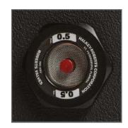
You'll also find a manual purge valve, so air pressure in the case can be equalised to the atmosphere. This prevents vacuumlock that can make opening the case
