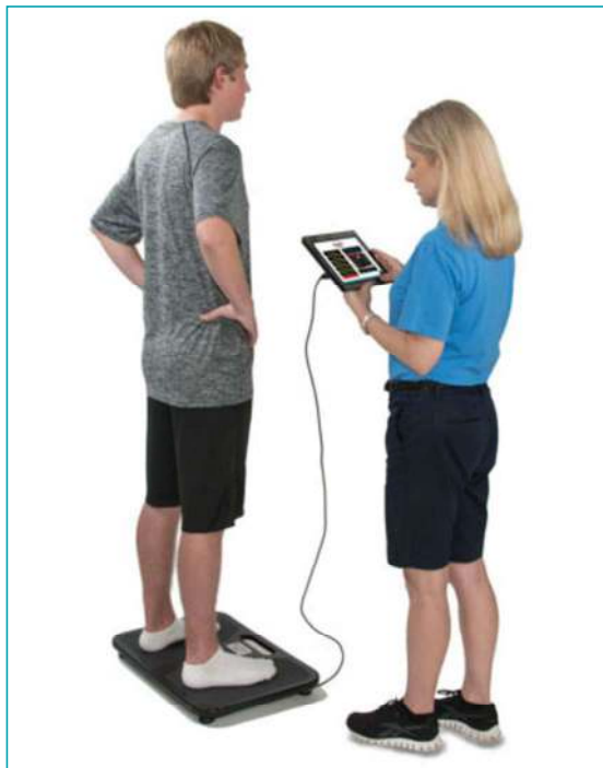
Figure 2 A depiction of typical BTrackS Balance Test administration. The athlete stands quietly on the BTrackS Balance Plate with eyes closed, feet shoulder width apart, and hands on hips, while the tester collects center of pressure information from the BTrackS Balance Plate using a computing device running BTrackS Sport Balance software. Photo from http://balancetrackingsystems.com/sport-balance , used with permission.
