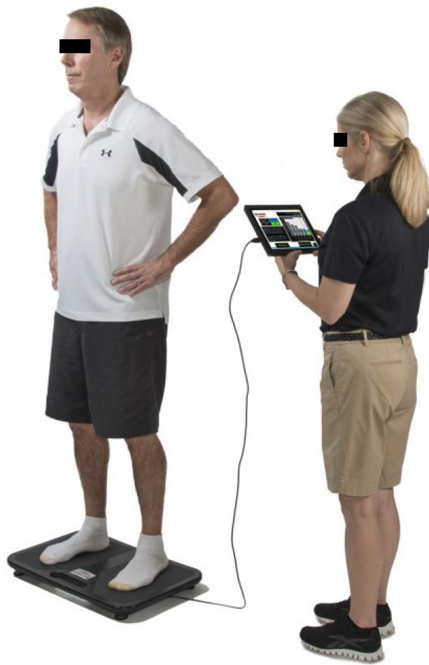
Figure 1 Depiction of BTrackS setup for postural sway testing. Participant stood on the BTrackS Balance Plate with feet shoulder width apart, hands on hips, and eyes closed for four 20 s trials. Postural sway was measured using the BTrackS Assess Balance software.
