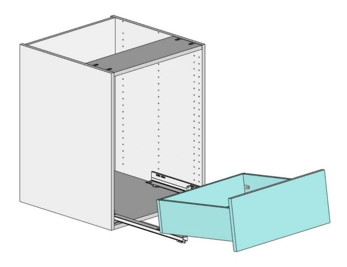
Pull the Drawer Guides out from the cabinet and align the DrawerBOX onto each of the guides. Push back into place until you hear a "click" sound.
