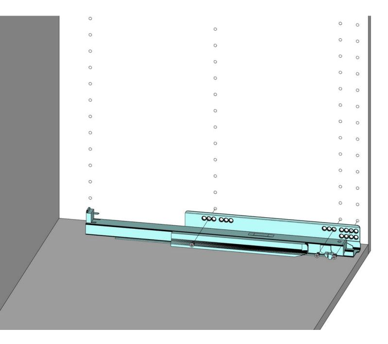
For a bottom-positioned standard DrawerBOX, align your Drawer Guides with the first row of holes. With the euro screws provided, screw through the Drawer Guides holes 2, 5, and 12 into the cabinet gable.
