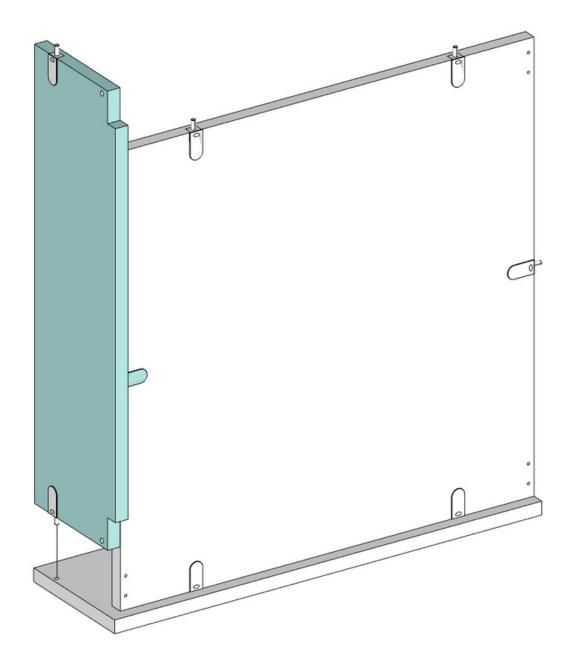
Attach the Drawer Back (KPDBA) to the Drawer Side (KPDSD), then, tighten the bottom fixing to the drawer back.
