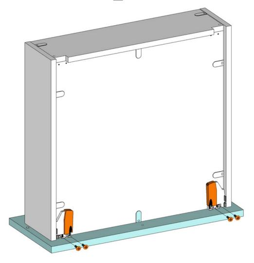
Tighten the Bottom (KPDBO) to the Drawer Front (KPDF). If you are assembling an Inner DrawerBOX, repeat this step with the Inner Front (KPIDF).
