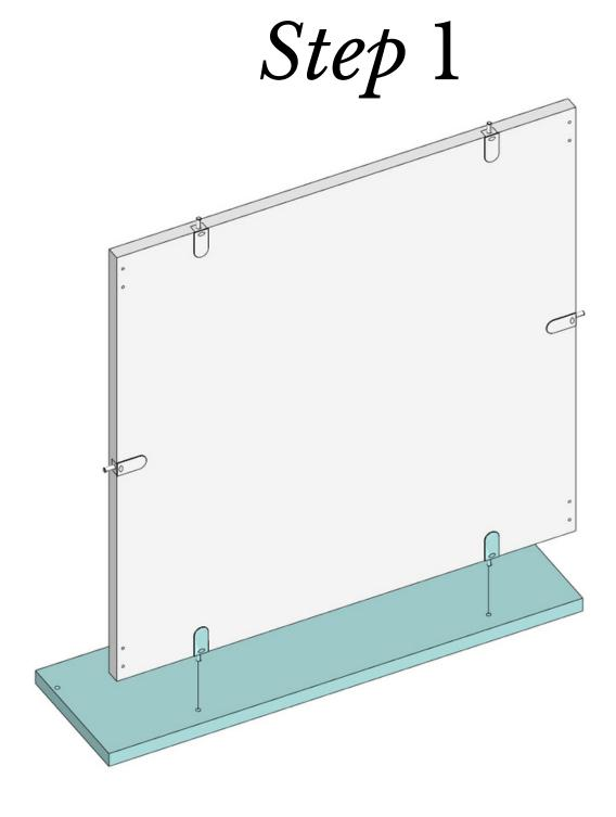
Attach the Drawer Bottom (KPDBO) to a Drawer Side (KPDSD) using the Kitch Assembly Tool.
