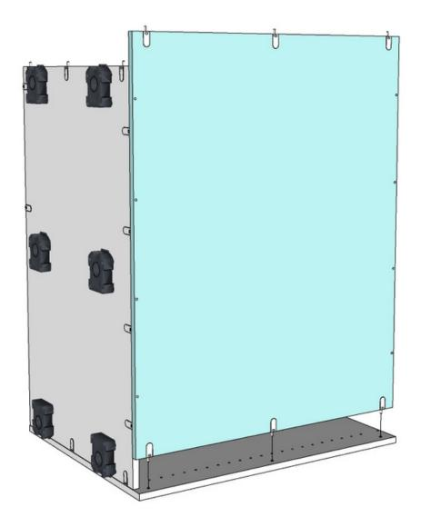
Attach the Back (KPBA) to the side Gable (KPGA), then, tighten the bottom fixings to the back.
