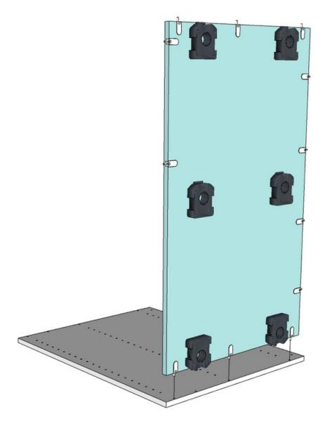
Attach the Bottom (KPBO) to the side Gable (KPGA) using the Kitch Assembly Tool.
