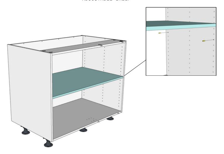
Insert the Adjustable Shelf Pins into the desired height location, then, place the Shelf (KPAS) on top of the pins.
