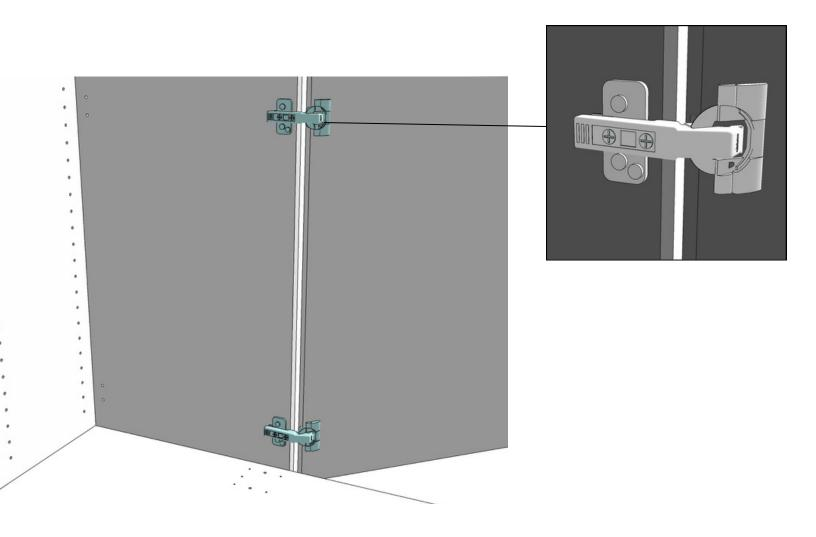
Attach the Door (KPDO) onto the hinge plate on the Blind Panel (KPBP) and click into place. Adjust the door as required.
