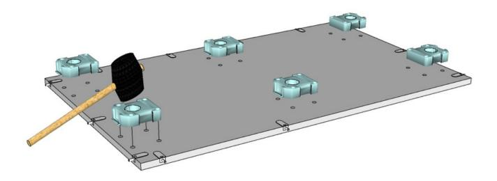
Attach the leg bases to the Bottom (KPBO).
