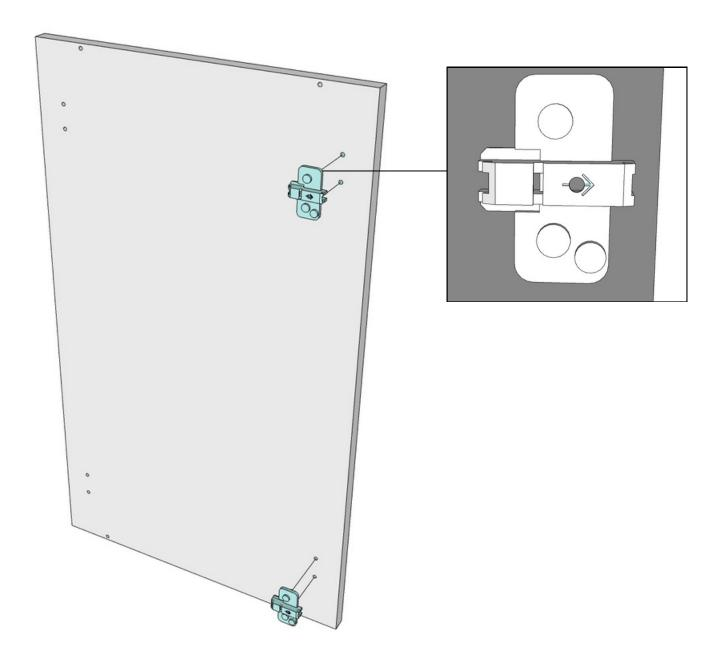
Attach the hinge plates to the Blind Panel (KPBP).
