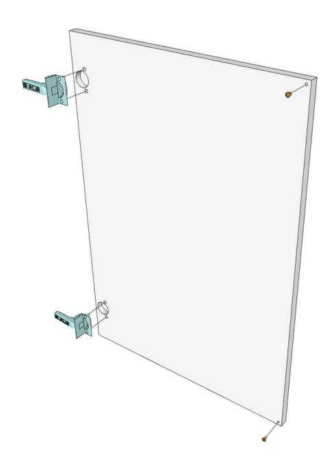
Attach the Blind Corner hinges to the Door (KPDO) and insert the bumpers.
