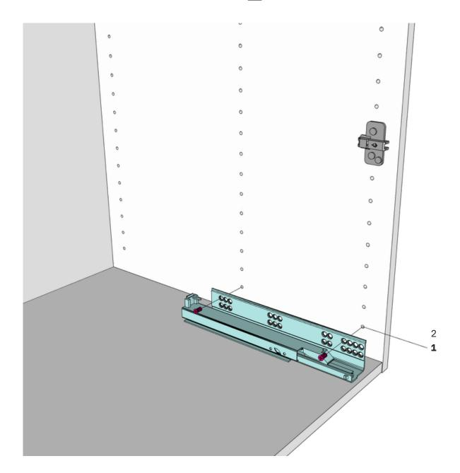
Align each Drawer Guide with the corresponding hole numbers on each Gable (KPGA). With the Drawer Guide Screws provided, screw through the Drawer Guide holes 4 & 12 into the cabinet gable.
