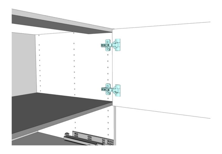
Attach the Door/s (KPDO) onto the hinge plates on the Gable (KPGA) and click into place. Adjust the door/s as required.
