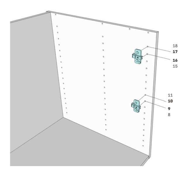
Insert the hinge plates into holes 9 & 10 and 16 & 17 of the side Gable (KPGA).
