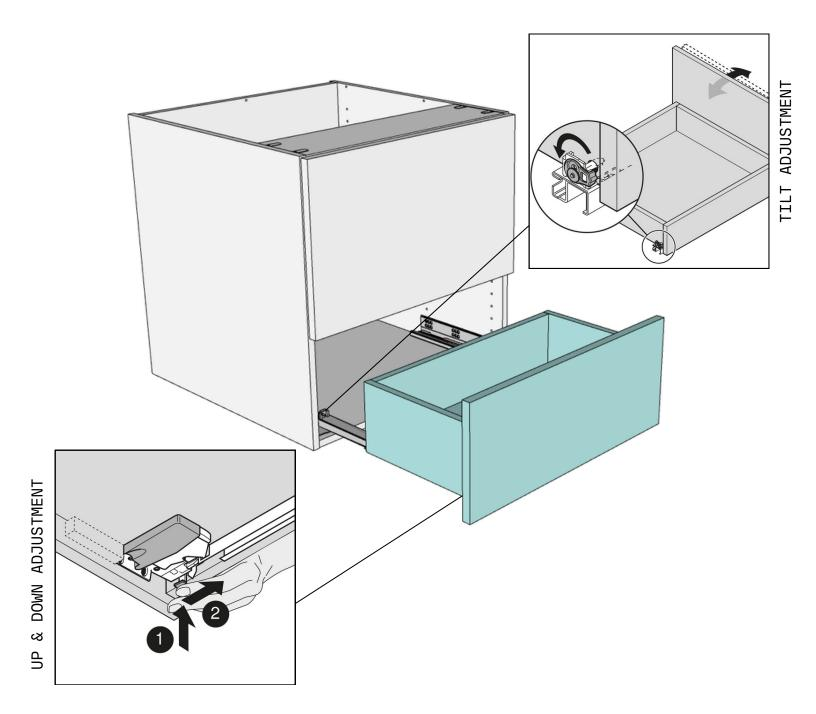
Pull the Drawer Guides out from the cabinet and align the DrawerBOX onto each of the guides. Push back into place until you hear a "click" sound.
