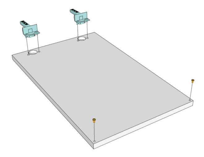
Attach the hinges to the Door/s (KPDO) and insert the bumpers.
