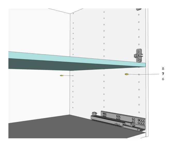
Insert the Adjustable Shelf Pins into hole 7, front and back, then, place the Shelf (KPAS) on top of the pins.
