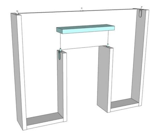
Attach the Inner Sink Front (KPIDF) to the Drawer Sides (KPDSDLO12LH & RH).
