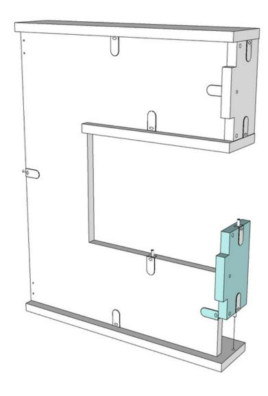
Attach the other Drawer Back (KPDBALO) to the Left Hand Drawer Side (KPDSDLO18LH), then, tighten the bottom fixing to the drawer back.
