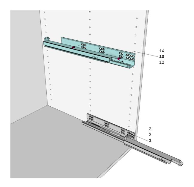
Align each Drawer Guide with the corresponding hole numbers on each Gable (KPGA). With the Drawer Guide Screws provided, screw through the Drawer Guide holes 4 & 12 into the cabinet gable.
