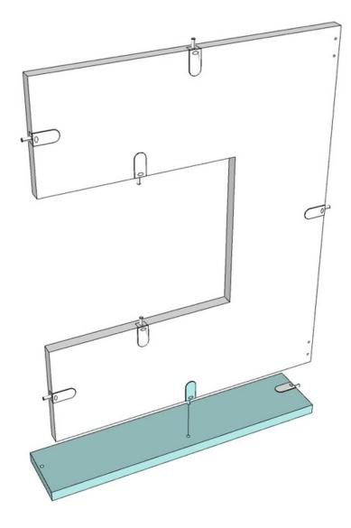
Attach the Sink Drawer Bottom (KPDBOSW) to the Right Hand Drawer Side (KPDSDLO18RH) using the Kitch Assembly Tool.
