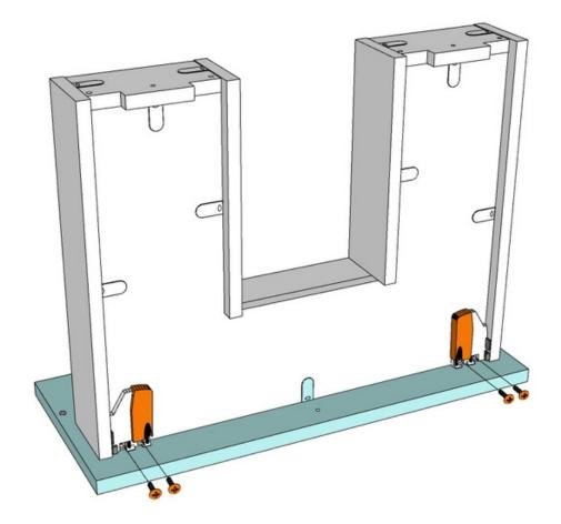
Tighten the Bottom (KPDBOSW) to the Drawer Front (KPDF).
