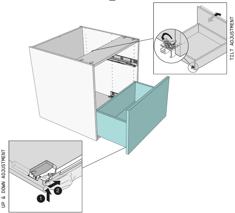
Pull the Drawer Guides out from the cabinet and align each DrawerBOX onto each of the guides. Push back into place until you hear a "click" sound.
