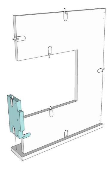
Attach one Drawer Back (KPDBALO) to the Right Hand Drawer Side (KPDSDLO18RH), then, tighten the bottom fixing to the drawer back.
