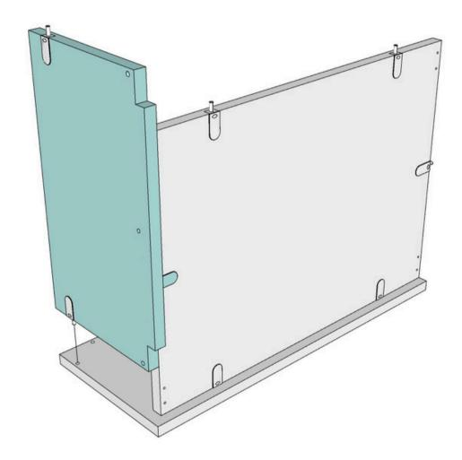
Attach the Drawer Back (KPDBA) to the Drawer Side (KPDSD), then, tighten the bottom fixing to the drawer back.
