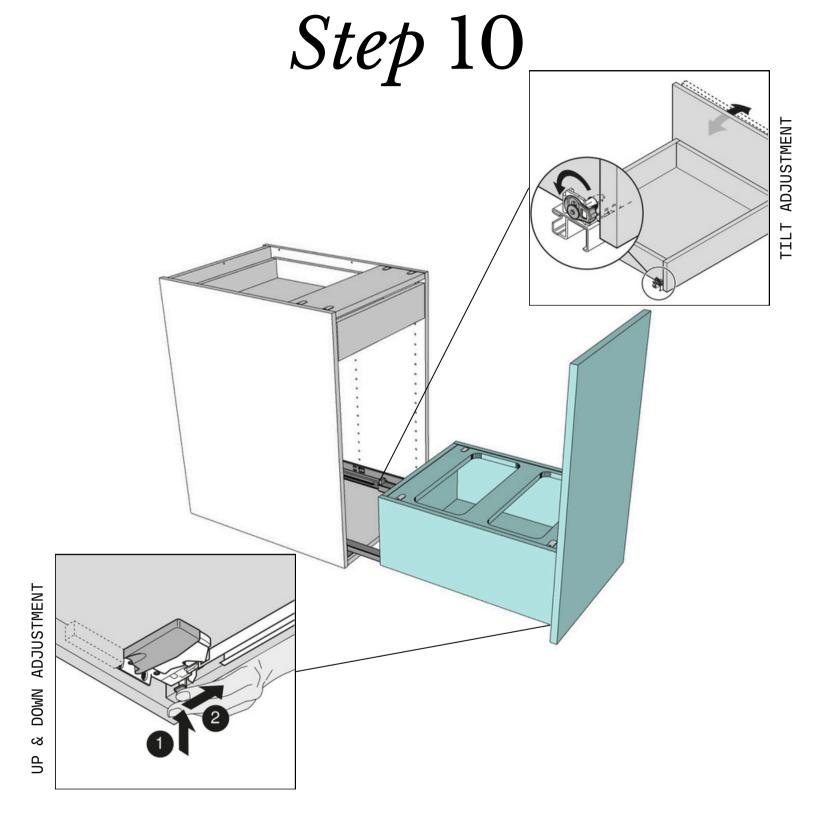
Pull the bottom Drawer Guides out from the cabinet and align the High Bin DrawerBOX onto the guides. Push back into place until you hear a "click" sound.
