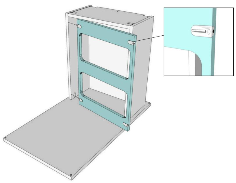
On the right side of the Garbage Drawer Bottom (KPDBO1822GR), unscrew both fixings so that the thread is flush with the edge of the panel, then, tighten the left side fixings to the left Drawer Side (KPDSD) followed by the right side.
