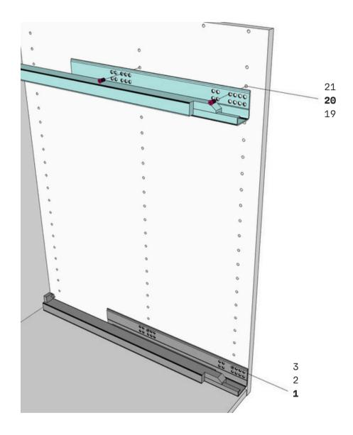
Align each Drawer Guide with the corresponding hole numbers on each Gable (KPGA). With the **Drawer Guide Screws** provided, screw through the Drawer Guide holes 4 & 9 into the cabinet gable.
