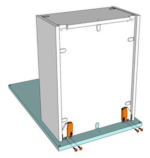
Tighten the Bottom (KPDBO) to the Drawer Front (KPDF).
