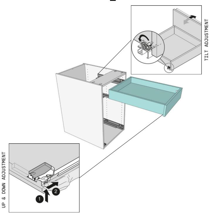
Pull the top Drawer Guides out from the cabinet and align the Inner DrawerBOX onto the guides. Push back into place until you hear a "click" sound.
