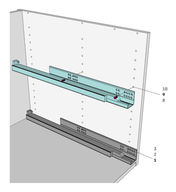
Align each Drawer Guide with the corresponding hole numbers on each Gable (KPGA). With the Drawer Guide Screws provided, screw through the Drawer Guide holes 4 & 9 into the cabinet gable.
