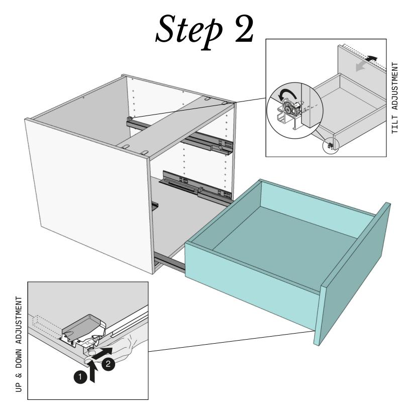
Pull the Drawer Guides out from the cabinet and align each DrawerBOX onto each of the guides. Push back into place until you hear a "click" sound.
