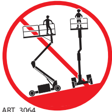
ART_3064 DO NOT ELEVATE OR DRIVE ELEVATED ON A SURFACE THAT EXCEEDS THE LEVELING RANGE
