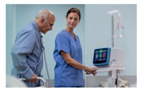
Our solution is **powered by AC with an internal battery** to add safety in the event of a power failure, a **transfer battery** for additional power needs, and has an **internal blower** that eliminates the need for air tanks during patient transfer.
